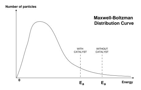
Lowering  $E_a$  results in there being a greater area under the curve showing that more molecules have energies in excess of the Activation Energy
