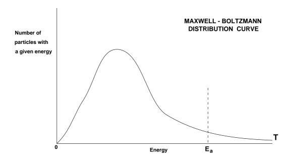
Significance E<sub>a</sub> corresponds to the **Activation Energy**. The area under the curve beyond this value is proportional to the number of particles with energy greater than E<sub>a</sub>
