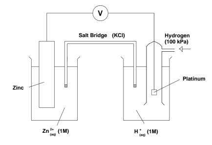
salt bridge • filled with saturated potassium chloride solution
