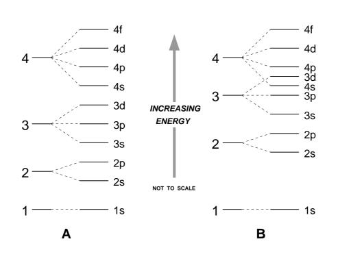
The diagram helps explain why the 4s orbitals are filled before the 3d orbitals
